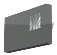
The cover is designed as a fixed shield for AM 900 when intake and exhaust air are closely located. The cover protects against external short circuits, by separating intake in the bottom of the cover and exhaust by the vertical grille in the front.
