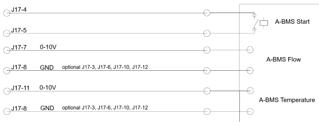
Figure 24: Analog BMS, AQC-L
