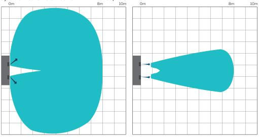
$<sup>^{10}</sup>$  The throw is measured with 2°C subcooled supply air.  $^{11}$  Set point for throw length can be adjusted using a PC with "Airling® Service Tool" installed.
