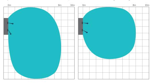
Asymmetrical air distribution<sup>15 16</sup> with Adaptive Airflow<sup>™</sup> and right facing inlet air grilles.
