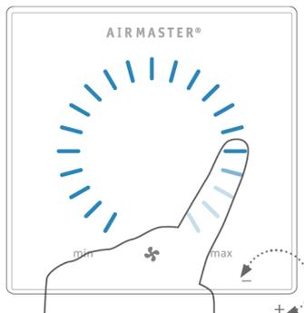
After 12 hours (time can be adjusted to 0, 1, 2, ... 255 hours using a PC running Airlinq Service Tool) the unit will return to automatic operation.
