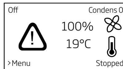
The Airmaster unit cannot be restarted until the cause of the alarm has been removed.
