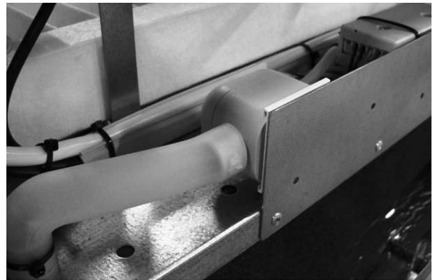
The condensate pump is available as an option and is therefore not supplied with all units. If the pump is fitted, its filter and the inlet pipe to the float chamber must be cleaned annually.
