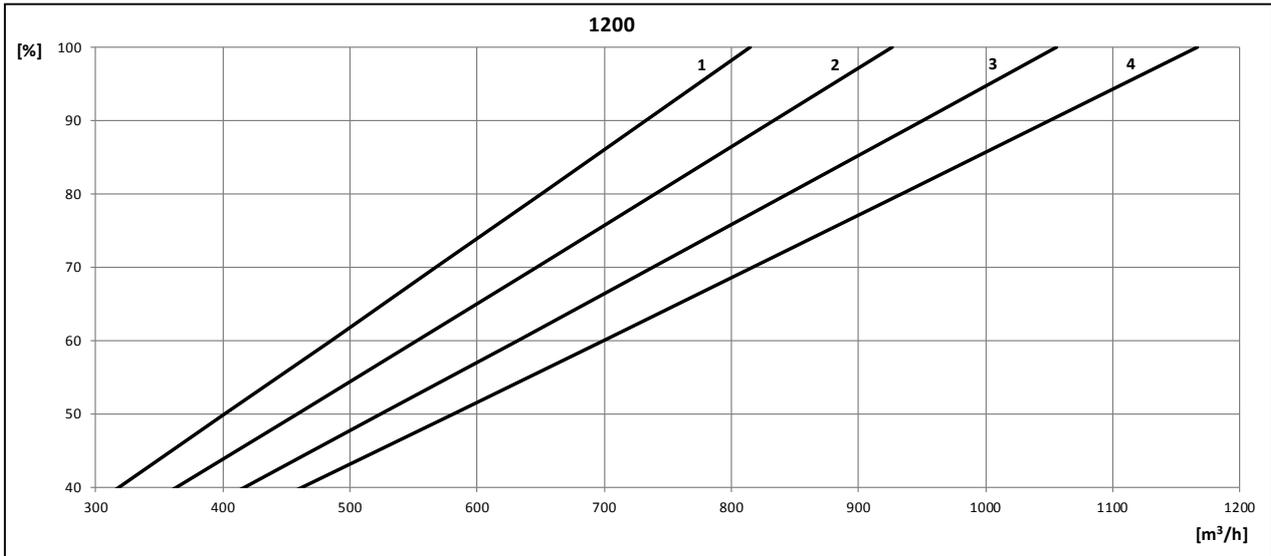
1: Corner, 30 dB(A); 2: Center, 30 dB(A); 3: Corner, 35 dB(A); 4: Center, 35 dB(A)
