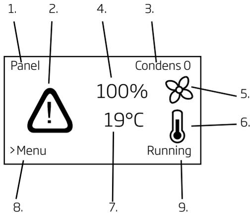
1. Activation - Indicates how the unit has been activated.
