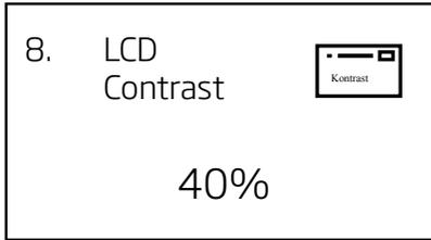
The contrast for the control panel display has been initially set at 40%. If you wish to change the contrast, this is set via the control panel as follows:
