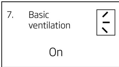
The basic ventilation function, which is activated and set via the control panel user menu, ventilates a room using a lower flow rate than is the case with general operation of the air handling unit.
