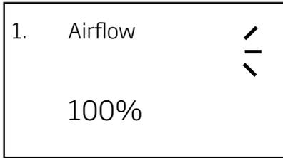
The airflow has been pre-programmed to a rate of 100%, but may be reduced right down to 40% (at CityVent 20%) in 1% steps:
