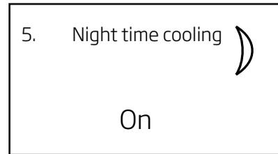
The night time cooling function, which is set via the control panel user menu, provides the option of reducing the room temperature overnight if the temperature has exceeded the nominal values during the day. The function works with a fixed parameter setting (high flow rate and low inlet temperature), which has been optimised to cool down the room's furnishings and structure to limit the room temperature during the day.
