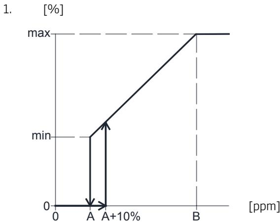
The unit starts with the programmed minimum airflow (min) when the CO<sub>2</sub> level exceeds the programmed lower limit plus 10% (A+10%). Depending on the CO<sub>2</sub> level in the room, the unit then increases the airflow in linear fashion until it reaches the maximum airflow (max) at the upper limit for the CO<sub>2</sub> level (B) and above.
