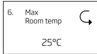
This menu item is hidden by default. The maximum room temperature may also be set via a parameter setting (for this, see section "3.5. Additional Parameters")
