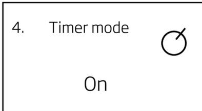
This function ensures fully automatic operation of the Airmaster air handling unit according to the programmed times.
