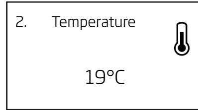
The inlet temperature is a setpoint for the temperature level of the unit. The default setting is 19°C. On units with/without a comfort heating surface, the temperature is set to the desired room temperature as a maximum/2°C below the desired room temperature.
